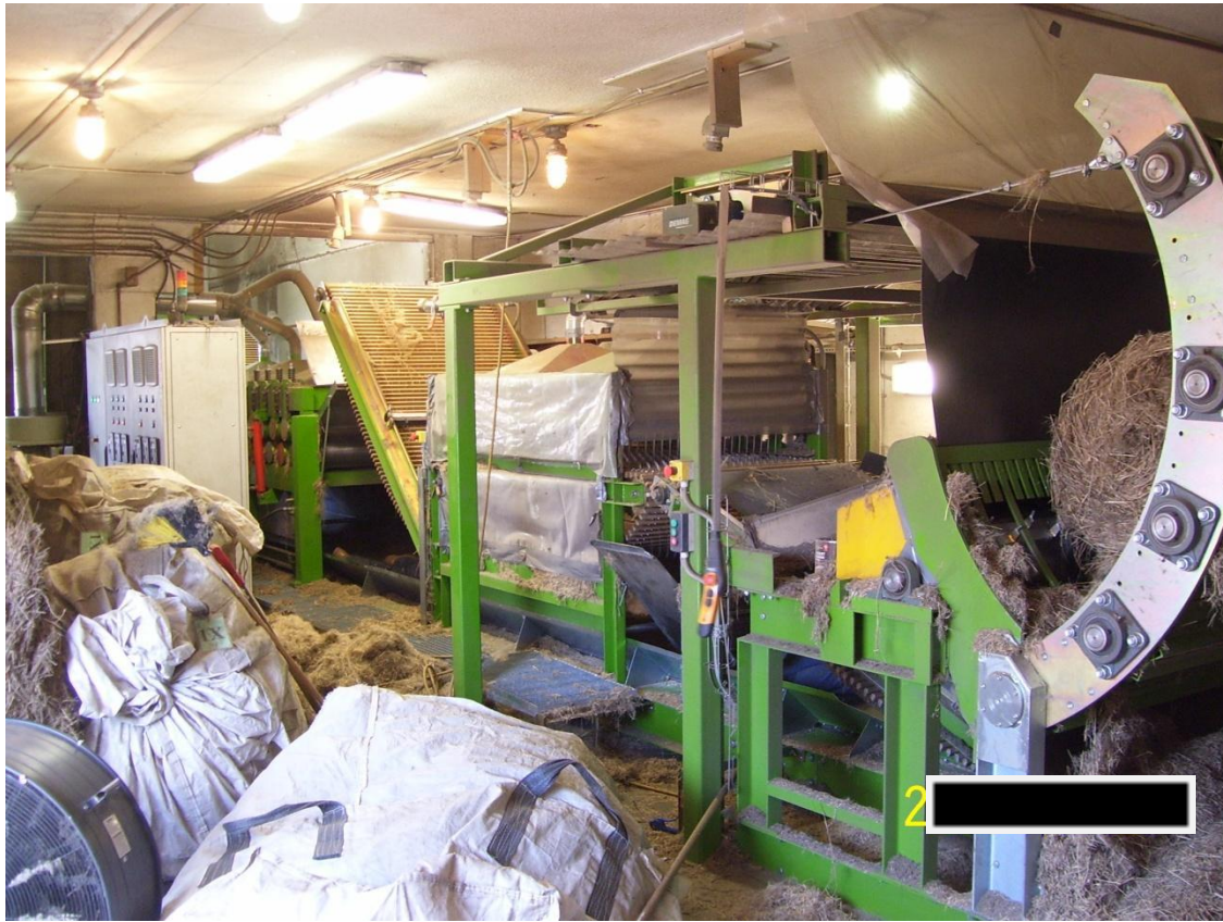
Figure 32 – The bale entry point of the Biolin Research flax straw and tow processing line
