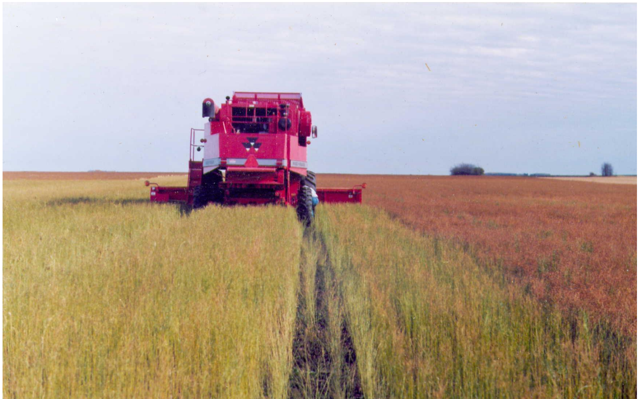
Figure 15 - Research into alternatives to "pulling" flax straw (using a stripper header on a combine to only harvest the seeds and leave the straw standing)
