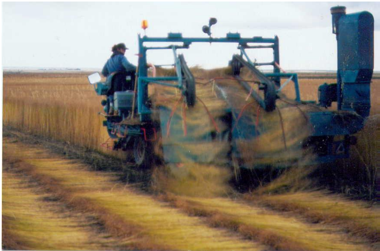
Figure 13 - Using a flax pulling machine to pull Saskatchewan grown fiber flax to copy what Europeans do to get high quality fiber
